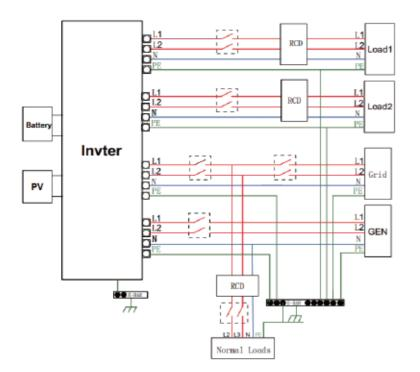
All switches and RCD devices in the figure are for reference only, and the specific installation shall be subject to local regulations.
